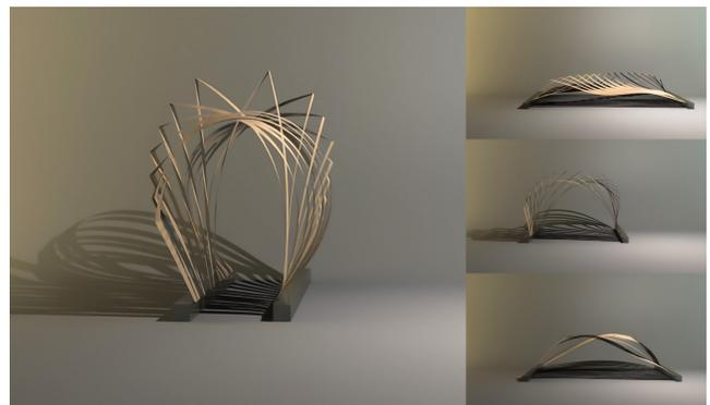
Figure 14: *Paper art*: A paper-art example assembled by ten paper strips with creases is simulated using 572 elements. The left ends of the strips are fixed, and the right ends move leftward to force the strips to pop upward. The right rows are middle frames of the simulation.
